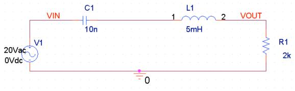
After you have completed this circuit, create a new simulation and change the analysis type to "AC Sweep/Noise".
