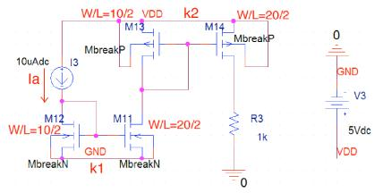
Here k1 and k2 is defined as the ration of the NMOS and PMOS respectively. We see that M11 is twice as big as M12 so k1=2, the same can be said for M13 and M14. So the current mirrored in through the resistor R3 will be  $I_axk_1xk_2$  (10uA\*2\*2 = 40uA).
