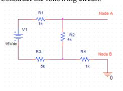
You can how ever always find the open circuit voltage Voc and short circuit current Isc by simulating each. To simulate a short circuit place a small resistor across node A and node B. For this example I used a 1 femto ohm. You should get Isc = 1.765mA for a short circuit current. For Voc replace the value with a large value, for this example I use 1 Tera ohm. Resulting with a Voc = 6V.
