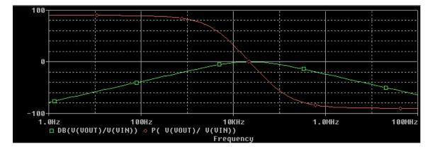
To plot the phase angle, we choose "P()" from the right column, and choose V(VOUT)/V(VIN). The resulting graph is shown above in red.
