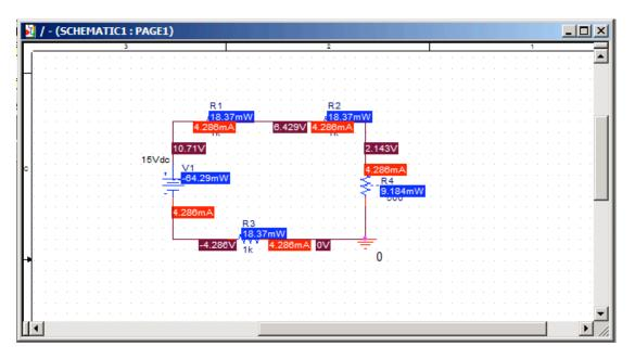
In blue is the power used by the element, in red is the current, and in maroon is the voltage.
