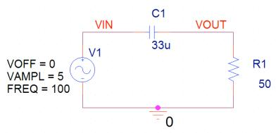
After constructing the circuit, create a new simulation profile. Since the frequency of V1 is 100Hz, the period is 0.01ms. So two periods will be enough for this simulation.
